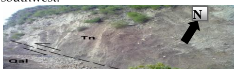
Photo 23: Shearing along the Bhalawal fault (Plate 2; station Banahal-1). Tn= Nagri Formation, Qal= Quaternary alluvium. Photograph facing southeast.
